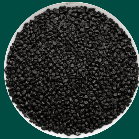
Granular Activated Carbon (GAC)
